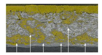
with **Dichtol** sealed ZnAl layer
